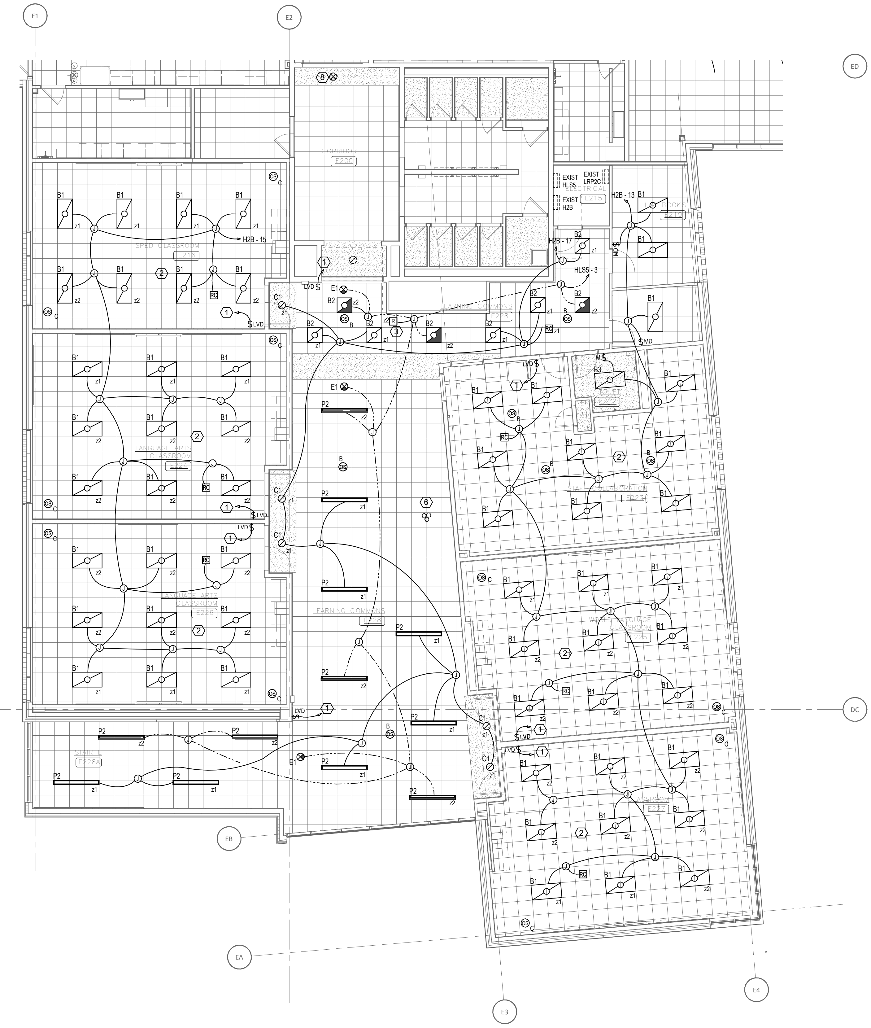
3 E200 SECOND FLOOR LIGHTING PLAN - AREA E SCALE: 1/8" = 1'-0"
